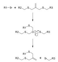
**Scheme 1.** Reaction mechanism for chain transfer within the polymer backbone.
